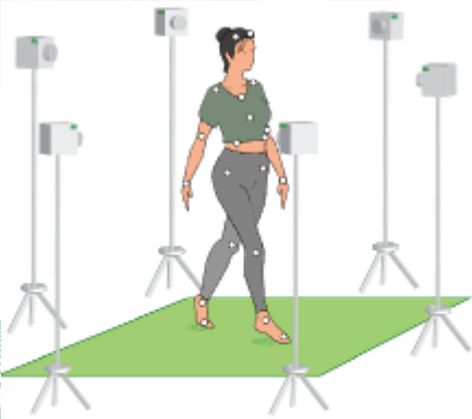
Optical motion capture using reflective markers
